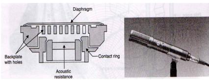
The fixed plate is mounted rigidly behind the diaphragm and in order to achieve as a high capacitance as possible very close to it. Capacitance can vary from 5 - 75 pF, but between 20 - 30 pF is most common.
