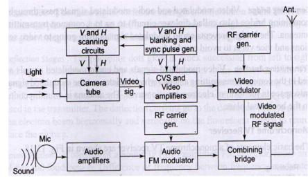
The basic elements of a monochrome TV transmitter are shown in the figure.
