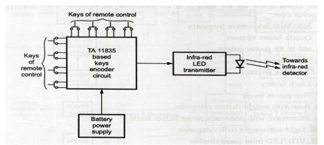
Most of the remote controls use single IC to perform all the operations. The ICS like TA 11835 etc are commonly used in remote controls. The circuit operates from small batteries or pencil cells. The remote control has single PCB and keypad. The keys of the remote control are interfaced to the IC based encoder. The contacts of the keys are printed on the PCB of the remote control. These contacts use carbon material. The pushbuttons or switches on the
