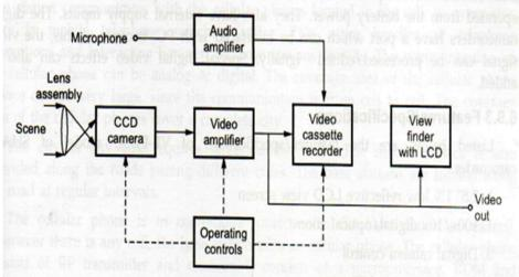
The lens assembly consists of zoom and focusing lens. This assembly is normally fitted with CCD camera. The CCD camera has auto focus facility. There id infrared transmitter and receiver in the camera. The infrared signals strike the scene / object in front of the camera. Based on the travelling time of the infrared signal, the distance of the scene / object is calculated. Then based on this distance, the focus is adjusted. The zoom lens is normally operated by the user.
