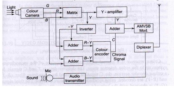
The basic features of a compatible colour transmitter are shown in the figure
