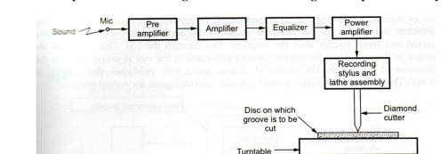
2) Draw and explain the Block Diagram of Disc Recording and Reproduction System.
